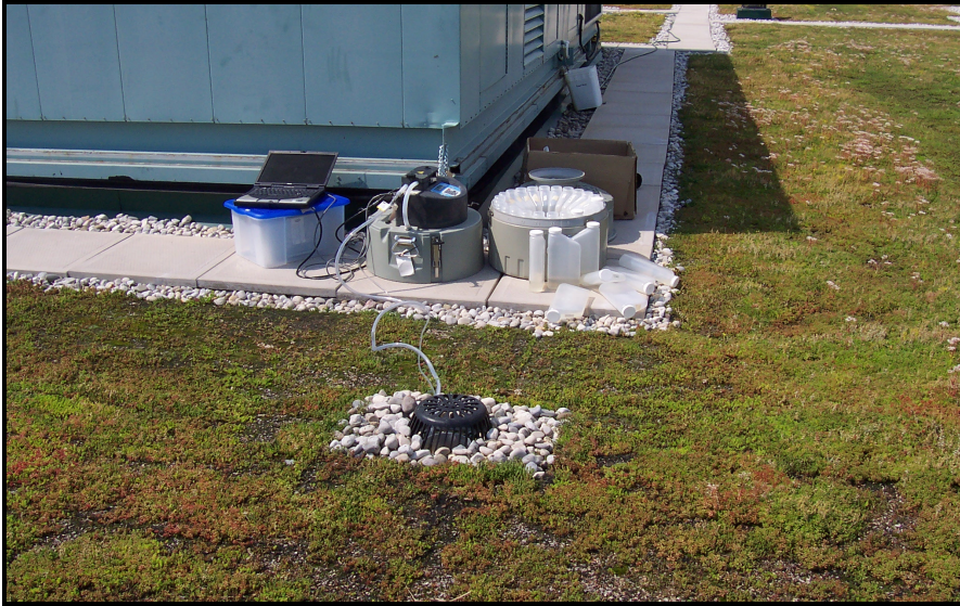
Figure 14: Water Sample and Data Collection with the ISCO 6700 Source: Vander Linden, 2006
