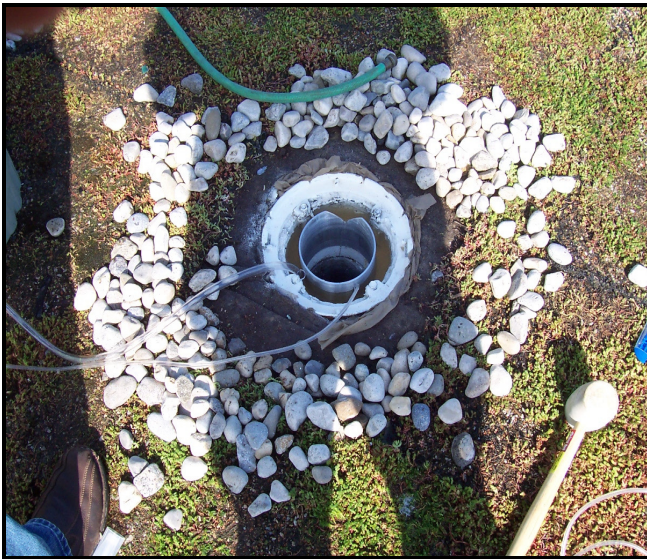
Figure 11: Green Roof Drainage Weir Source: Vander Linden, 2006
