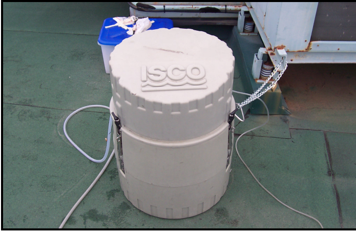
Figure 12: ISCO 6700 Automatic Sampler Source: Vander Linden, 2006
