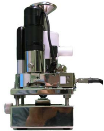
Figure 9. Atomic Force Microscope on translation stage with contact lens on glass sphere.
