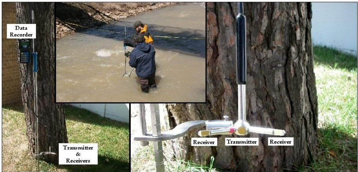
Figure 2-6. Example of 2D Acoustic Doppler Profiler.
