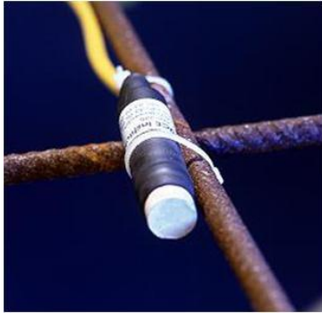
Figure 16: Embedded Mn-MnO 2 reference electrode (Klinghoffer)
