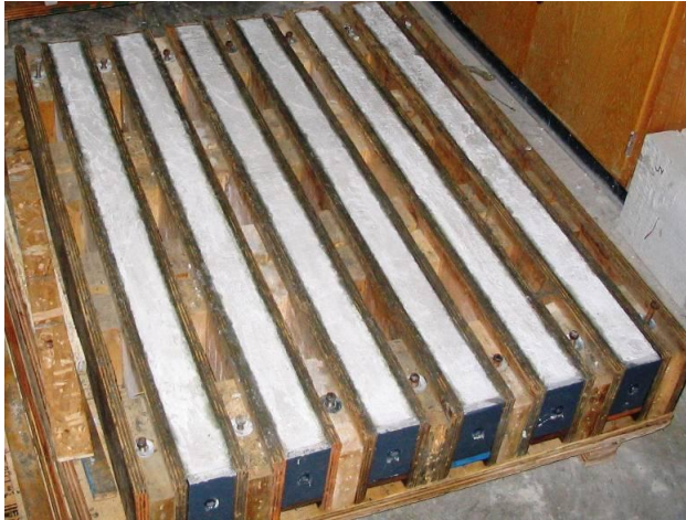
Figure 29: Loaded beams cast into formwork
