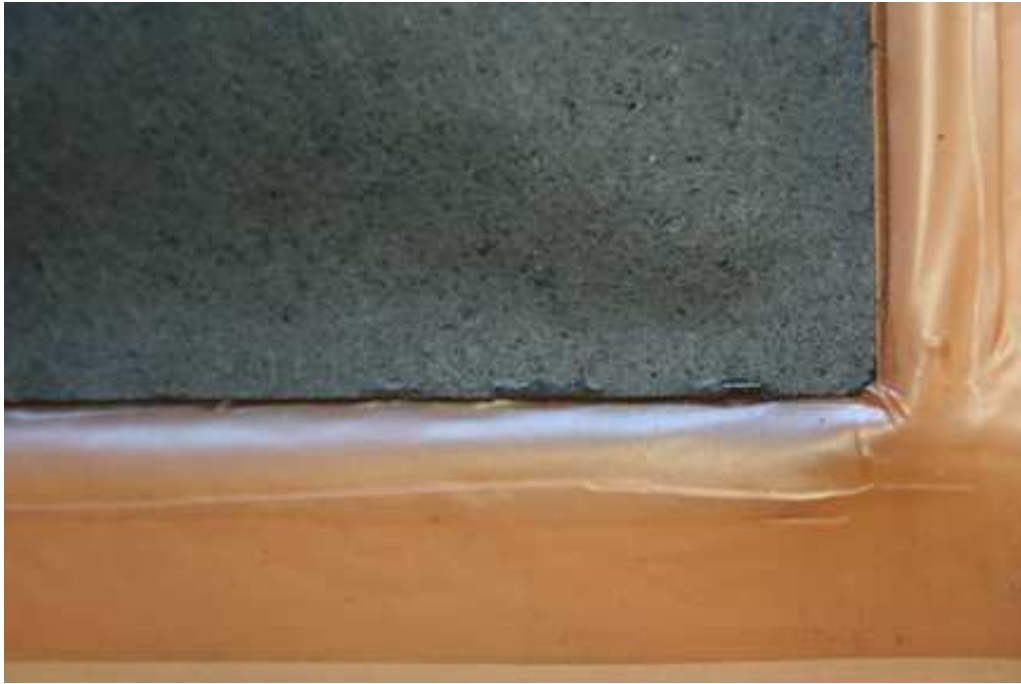
Figure 4.4: Damaged 5 layer MEA - 2
