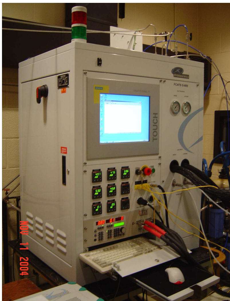
Figure 3.14: Hydrogenics' Fuel Cell Automated Test Station (FCATS)
