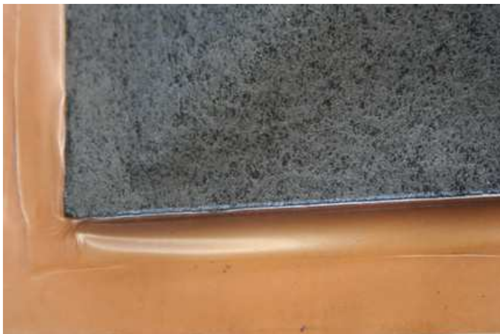
Figure 4.3: Damaged 5 layer MEA - 1
