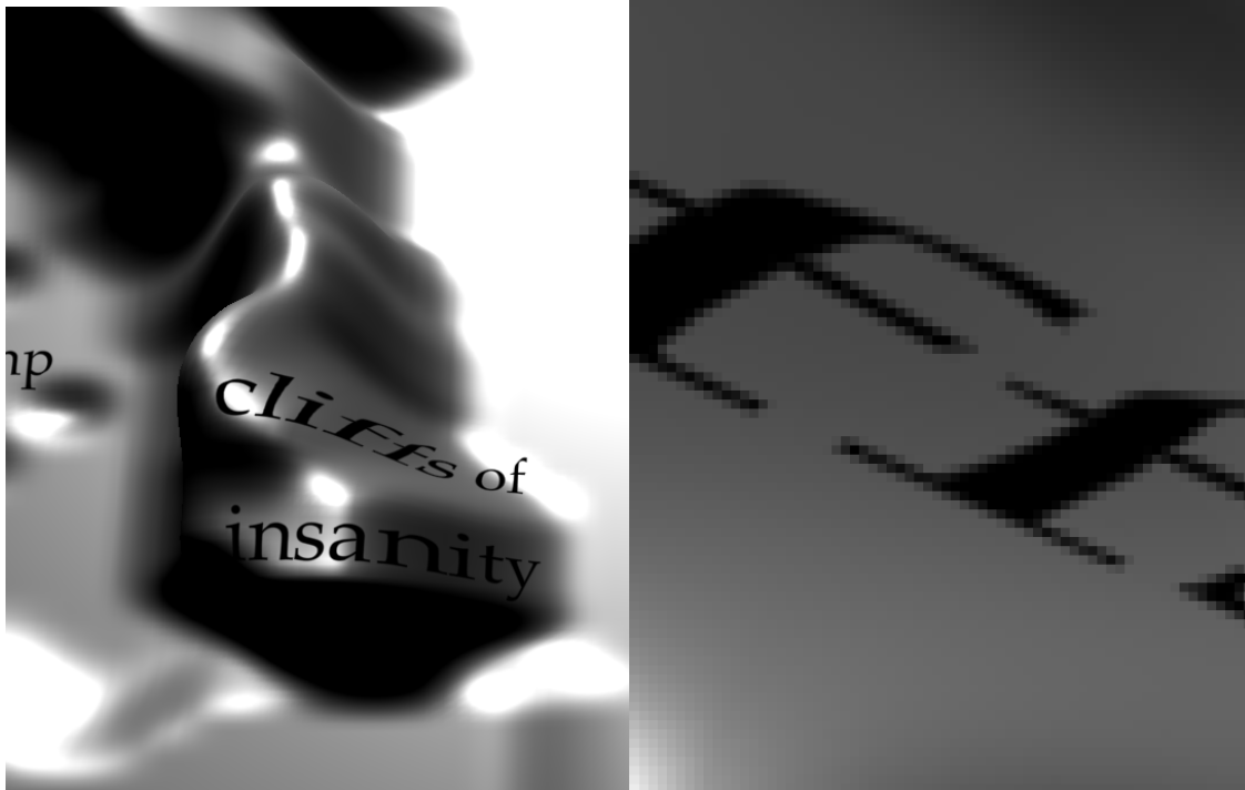
Figure 4.10: A map using a vector texture for labels, with an enlargement of a distorted region to demonstrate anisotropic antialiasing.
