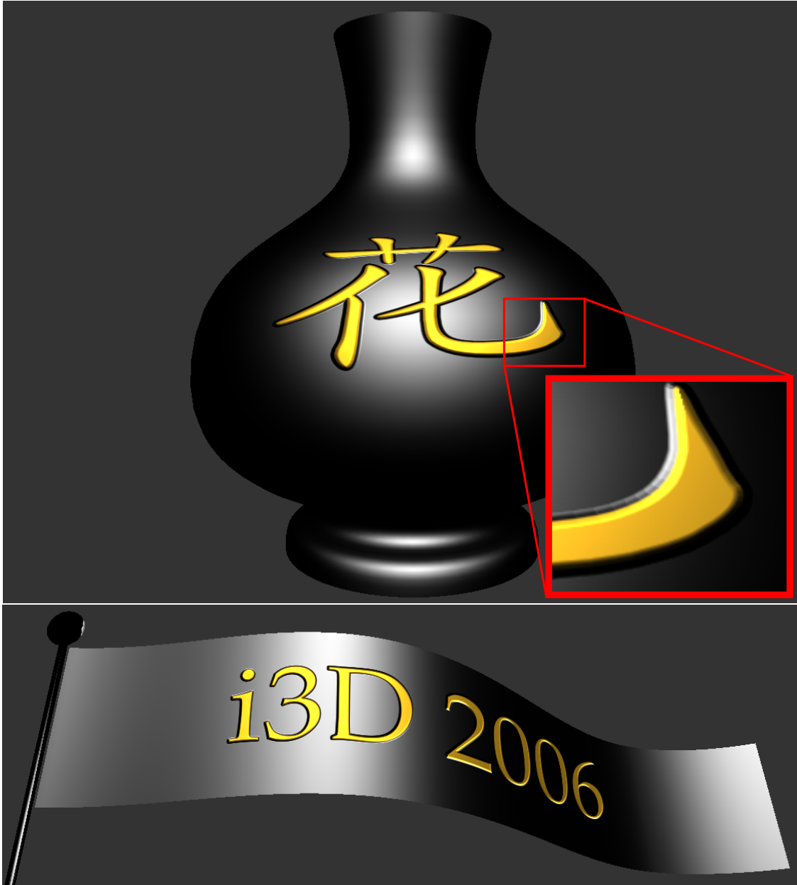
Figure 4.8: Some examples showing embossed glyphs. The gradient of the distance field is used to perturb the normal. In the top example, the inset image shows creases along line segment junctions when the glyph is magnified to a certain degree
