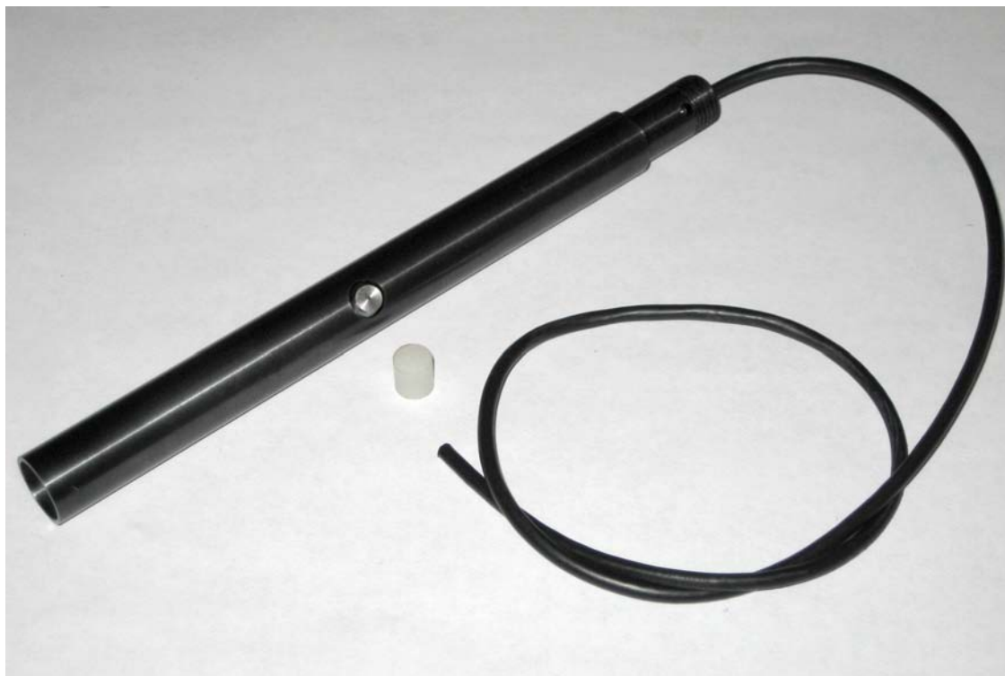
Figure 6.21: Test specimen showing nylon sleeve for near field pressure sensor.
