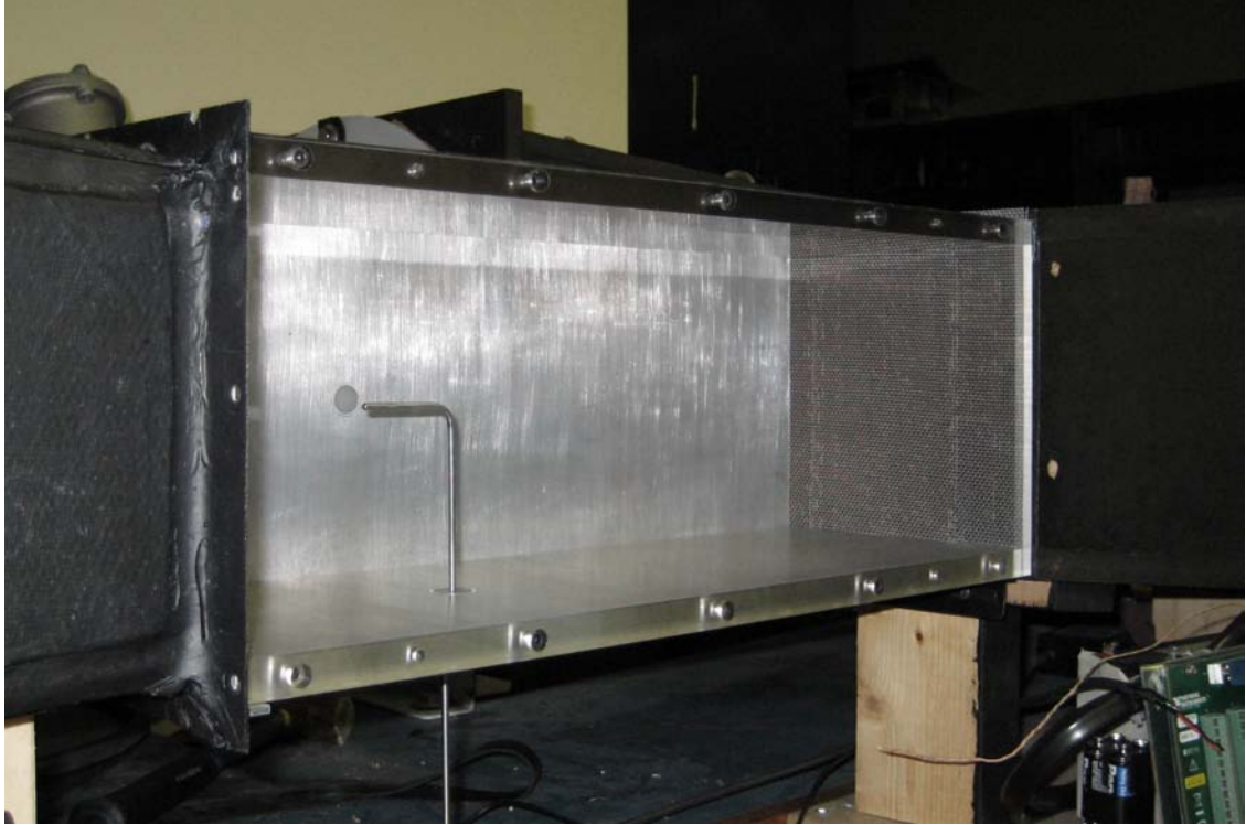
Figure 6.13: Screen installed at outlet of wind tunnel test section.
