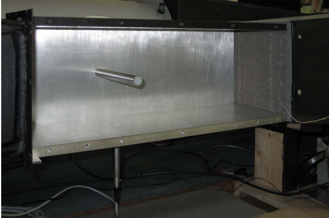
Figure 6.24: Test specimen installed in wind tunnel.
