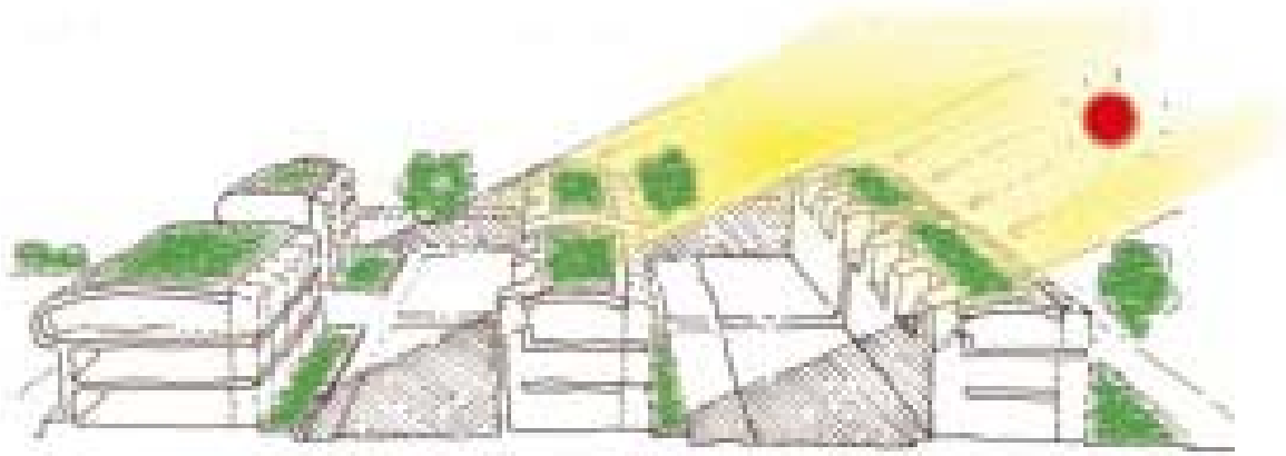
Figure 12 - schematic cross-section depicting form shaped by solar access at three stories as used in the design of BedZed in UK. (BedZed, 2008)
