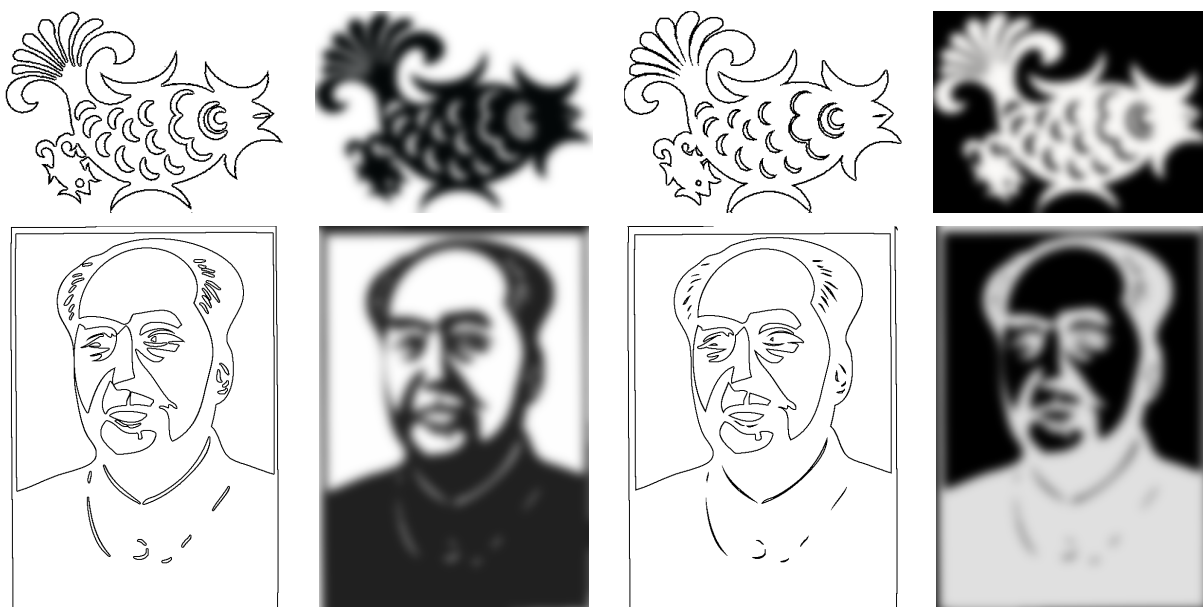
Figure 1.16: Spatial scales of images in Figure 1.15. Each image includes a high spatial frequency data (left) and low spatial frequency data (right). Tone inversion images have similar high spatial frequency data as original images. But low spatial frequency data are totally different.
