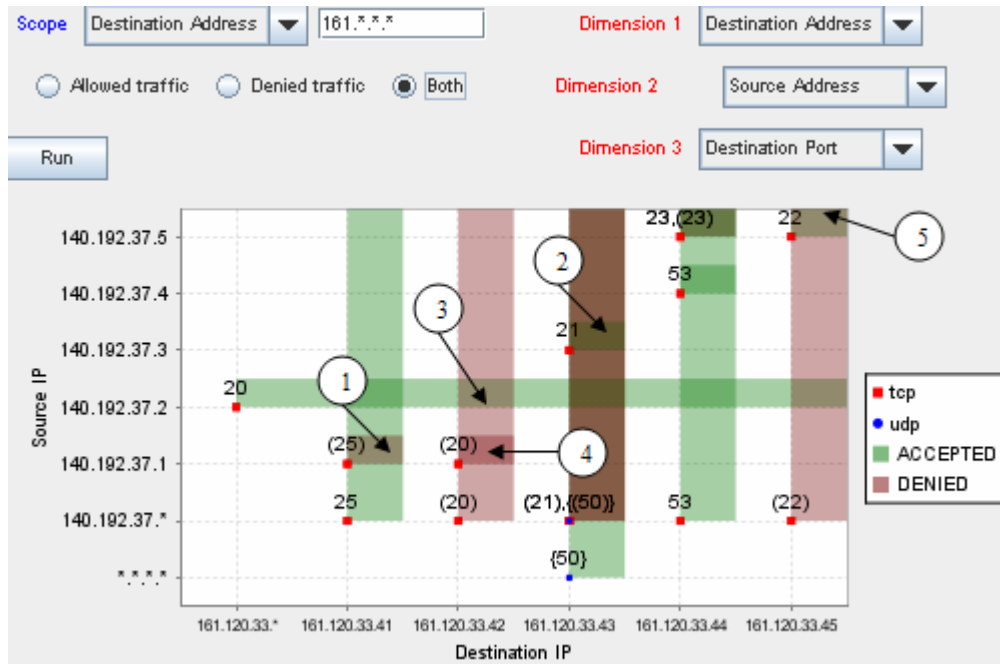
Figure 2.8. Many potential anomalies in the policy (these arrows are manually inserted)
