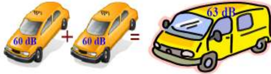
Figure 2-6 Sounds from Two Independent Sources (Ahammed and Tighe 2008c).
