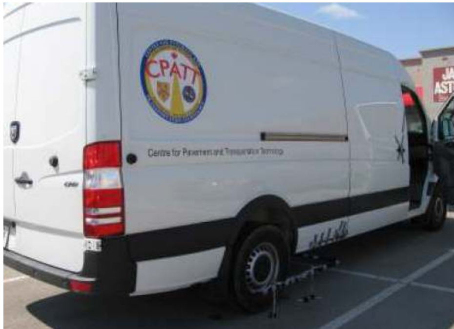
Figure 4-16 Physical Set-up for CPX Noise Measurement.
