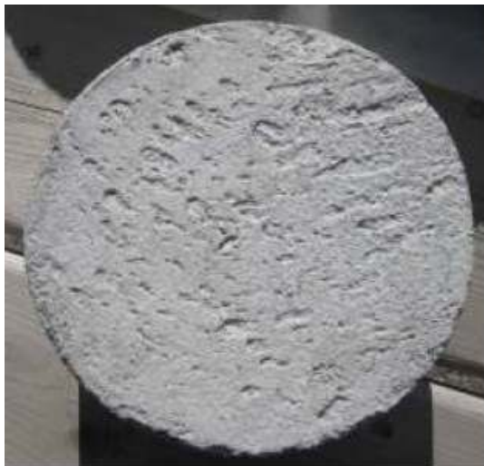
a) Screed Finish
