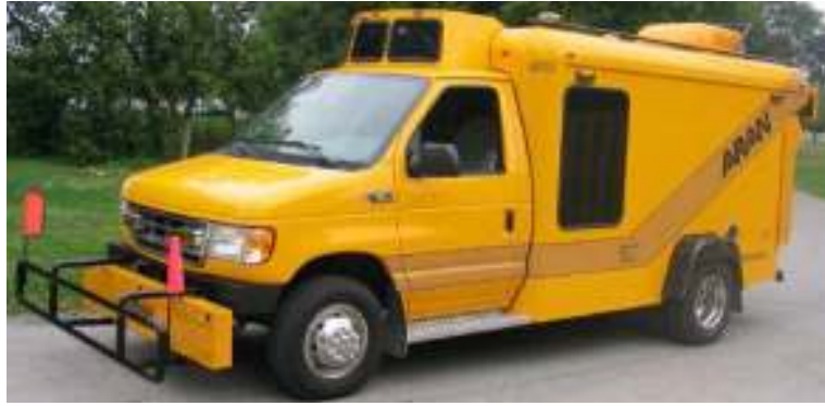
Figure 4-10 Automatic Road Analyzer (ARAN) (Courtesy: Roadware, Paris, Ontario).
