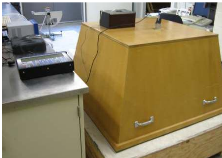
Figure 4-21 Sound Absorption Testing using Reverberation Chamber.
