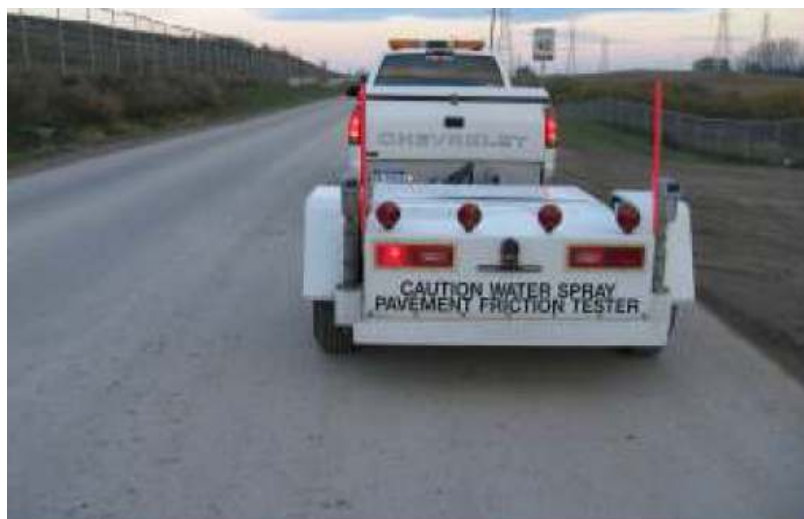
Figure 4-9 Skid Resistance Measurement with Dynatest Friction Tester.
