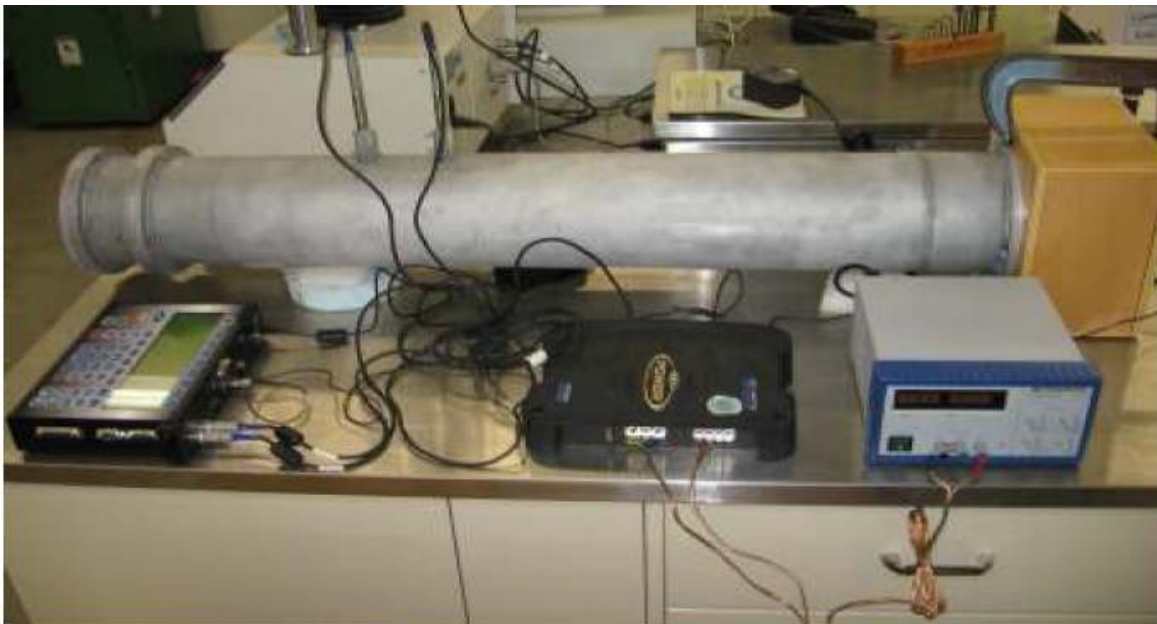
Figure 4-19 Impedance Tube for Sound Absorption Test at CPATT Laboratory.
