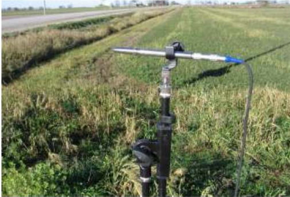
Figure 4-18 Physical Set-up for CPB Noise Measurement.
