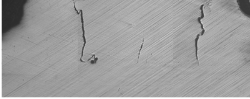
Figure 4.29 Isolated micro-cracks in cross-section of the thin wall at x = 12.5 mm with substrate preheated to 600 K
