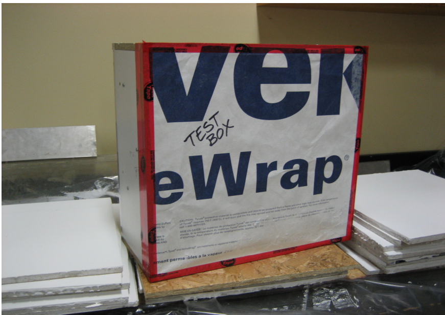
Figure 4-7: Test Box, After Tyvek Installed on Exterior Face
