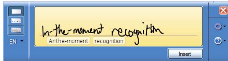
Figure 2.1: The pen input panel on a Windows XP Tablet PC. An example of in-the-moment recognition
