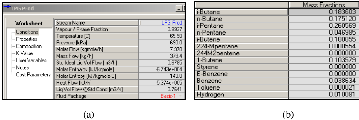
Figure 4.15 The LPG Product stream to storage tank: (a) conditions and (b) compositions.
