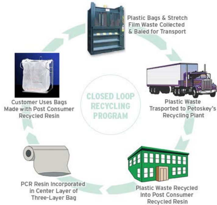
Figure 2-33: Diagram of the closed loop recycling process, where plastic bags and film are collected following their intended use and returned for recycling and reintroduction into the same market application.
