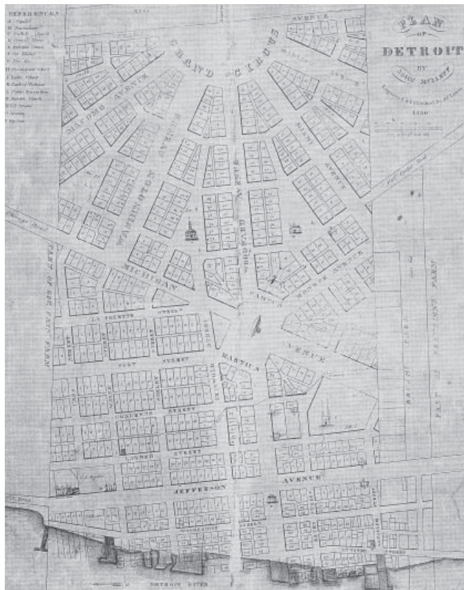
Figure 2.9. (Above) John Mullett’s plan of Detroit in 1830. This plan shows the portions of the Woodward plan that were carried out. The Woodward plan consisted of interlocking hexagons that consisted of large north-south and east-west boulevards that, when bisected would form large circular plazas or circuses. The plan was adopted in 1807 and abandoned in 1818.
