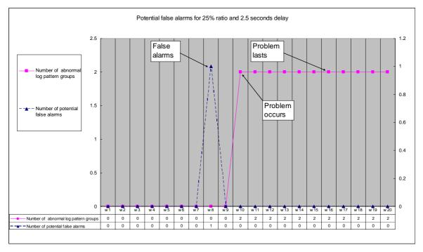
Figure 4.12: Number of potential false alarms for 25% ratio and 2.5 seconds delay
