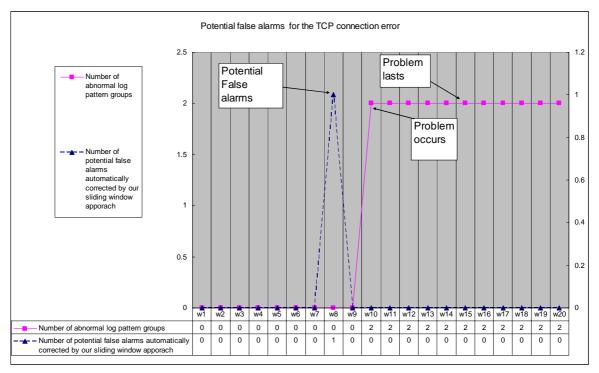
Figure 4.8: Potential false alarms automatically corrected for the TCP connection error
