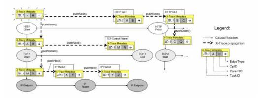
Figure 2.8: An example of propagation of metadata for a HTTP request[2]
