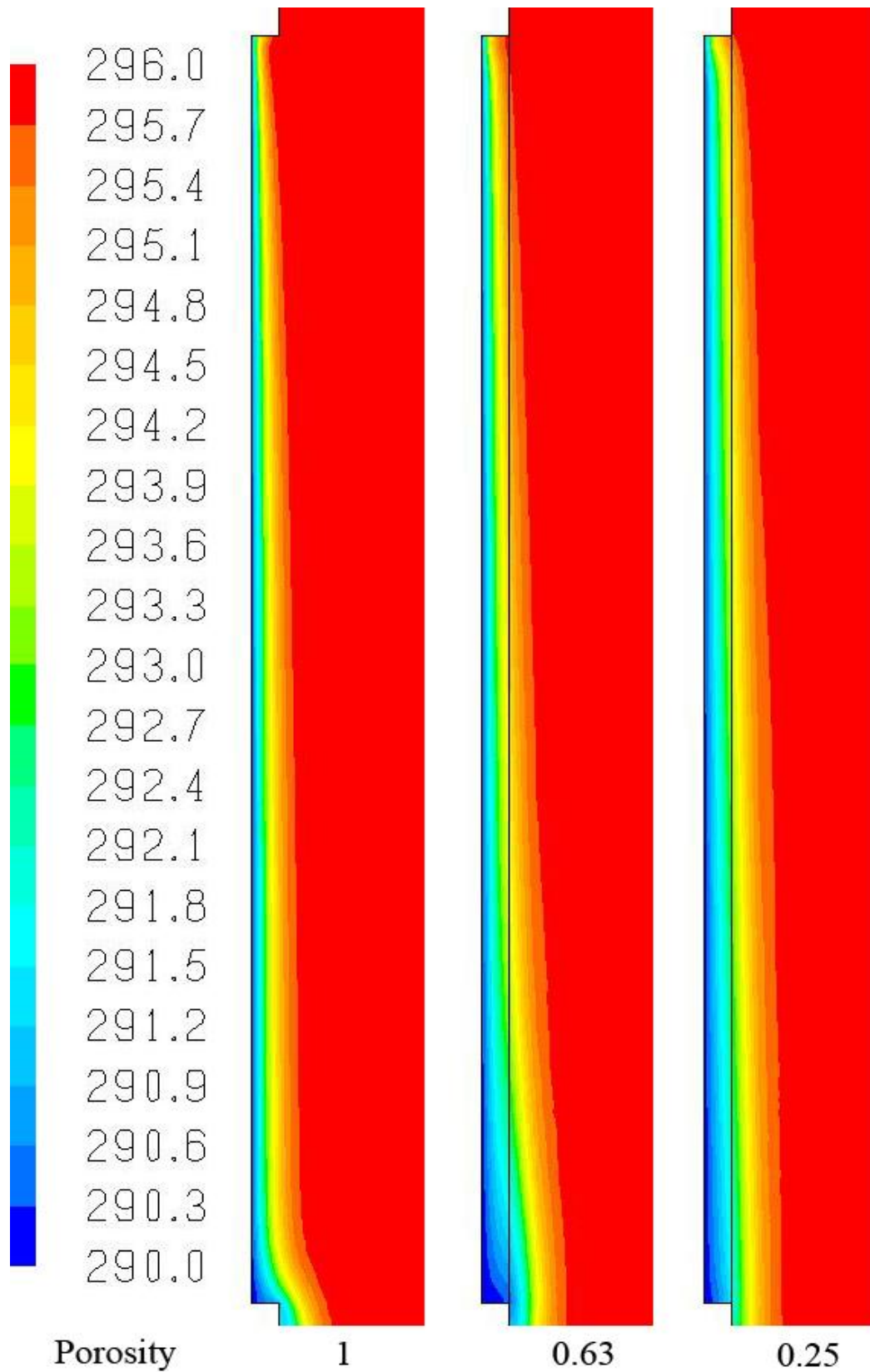
Fig.4.2. Temperature Plots in K for 0.6096m height, 0.0127m sill window with T_g = 290 , \gamma = 1.0 , 0.63, 0.25
