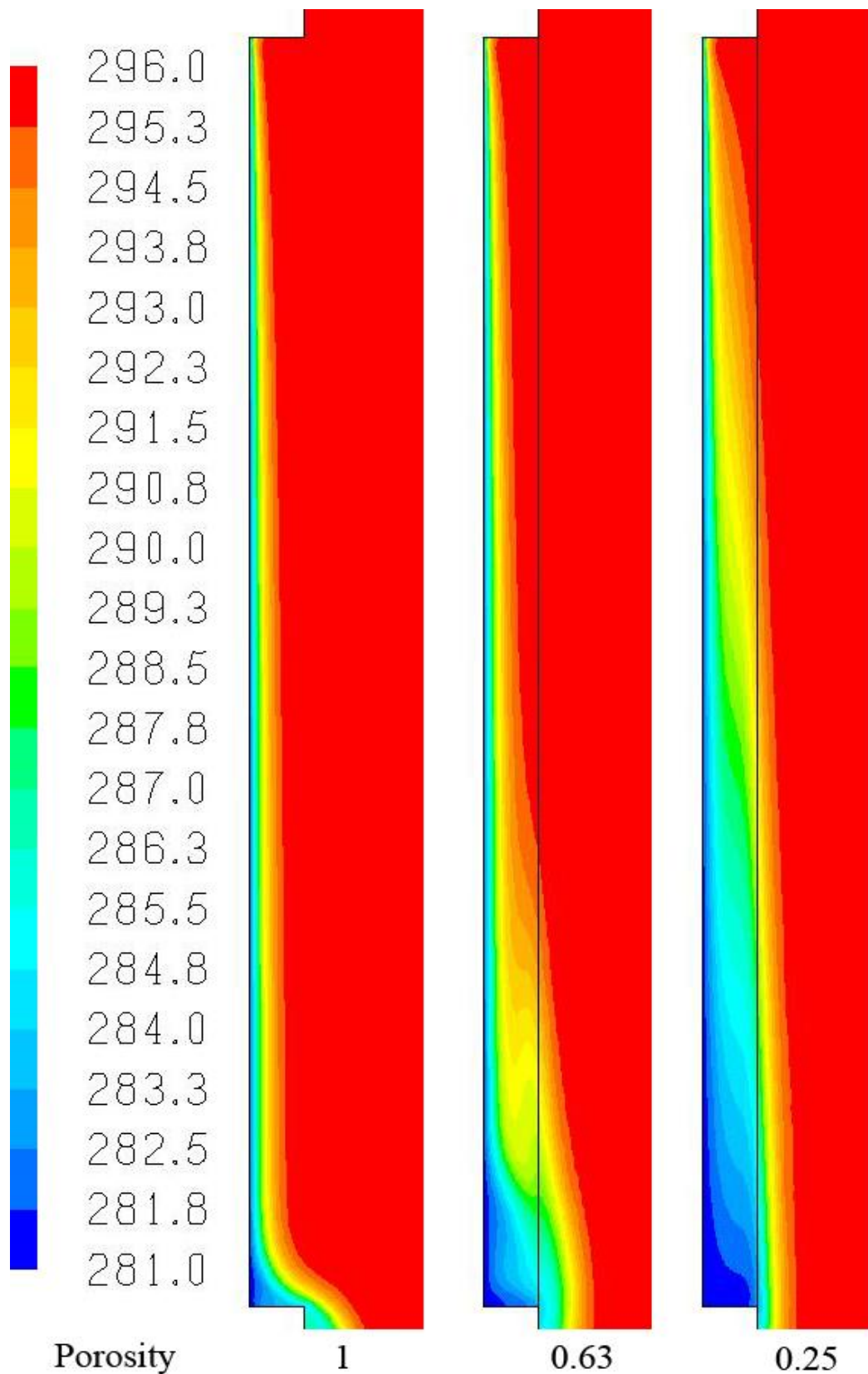
Fig.4.8. Temperature Plots in K for 0.6096m height, 0.0254m sill window with T_g = 281 , \gamma = 1.0 , 0.63, 0.25
