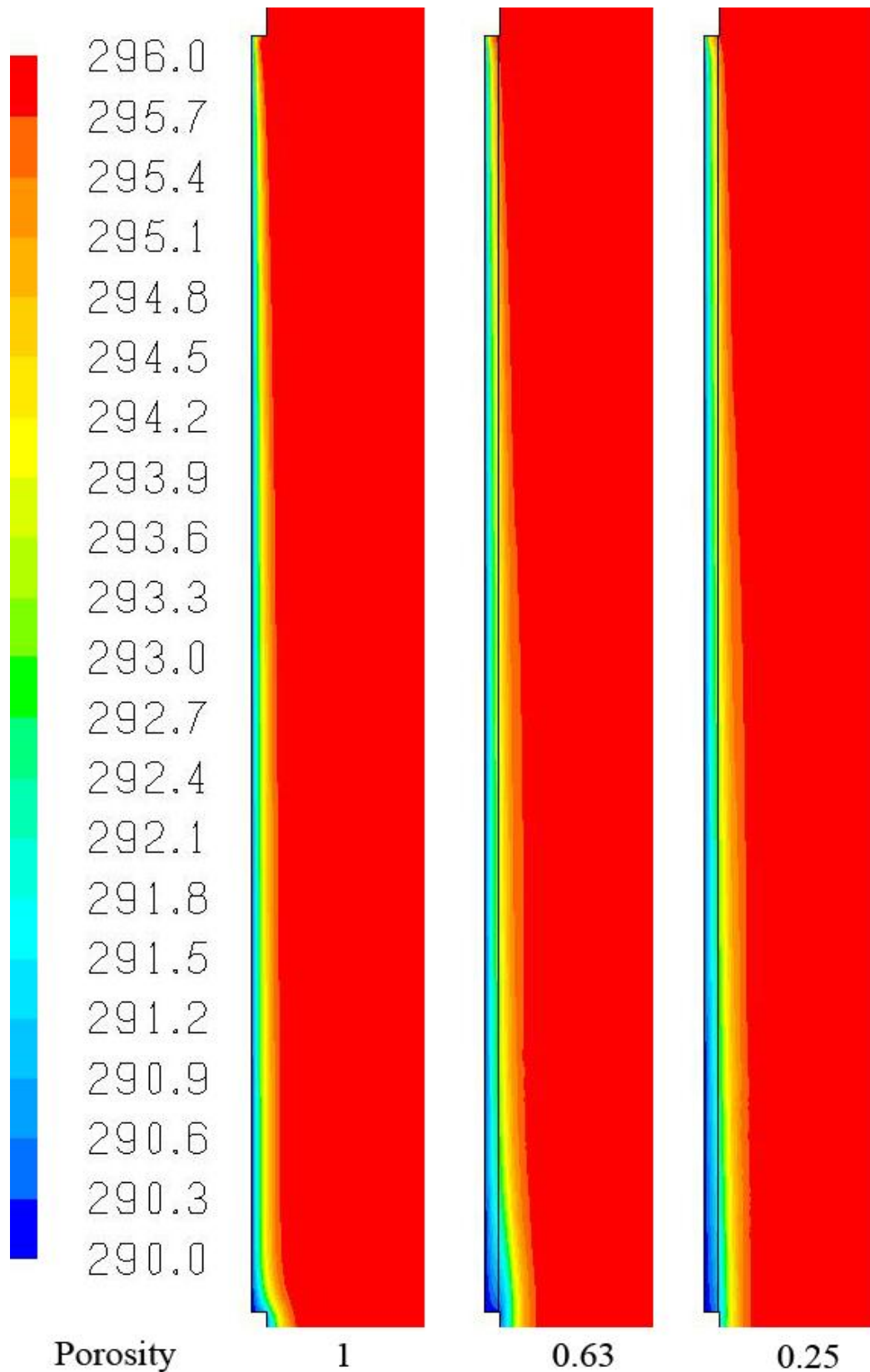
Fig.4.10. Temperature Plots in K for 1.22m height, 0.0127m sill window with T_g = 290 , \gamma = 1.0 , 0.63, 0.25
