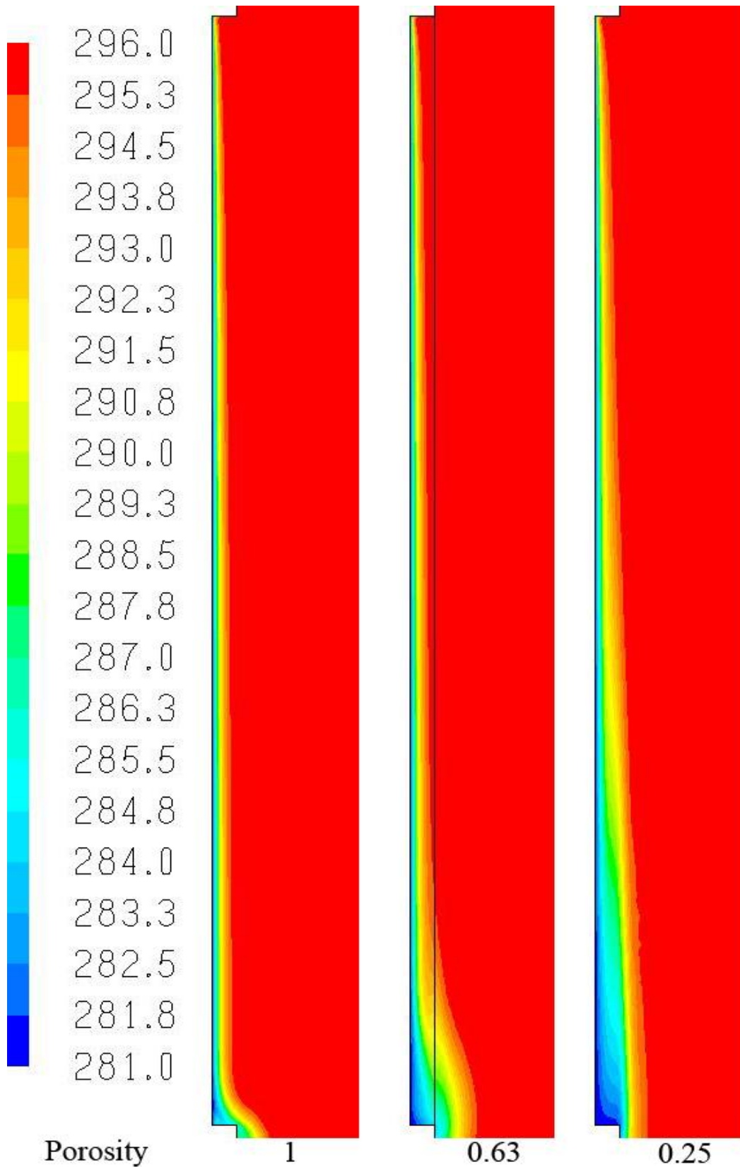
Fig.4.16. Temperature Plots in K for 1.22m height, 0.0254m sill window with T_g = 281 , \gamma = 1.0 , 0.63, 0.25
