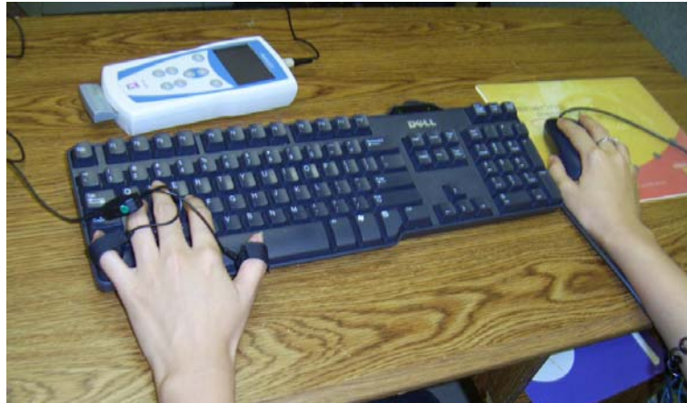
Figure 14: Left hand for controlling keyboard, collecting GSR data; right hand for controlling mouse.
