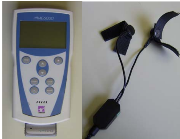
Figure 13: ME 6000 Biomonitor and its sensors for collecting GSR data
