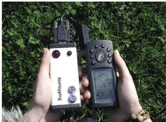
Figure 5: Device (GSR tester + GPS) used in Bio Mapping project (Original source: Nold, 2004)
