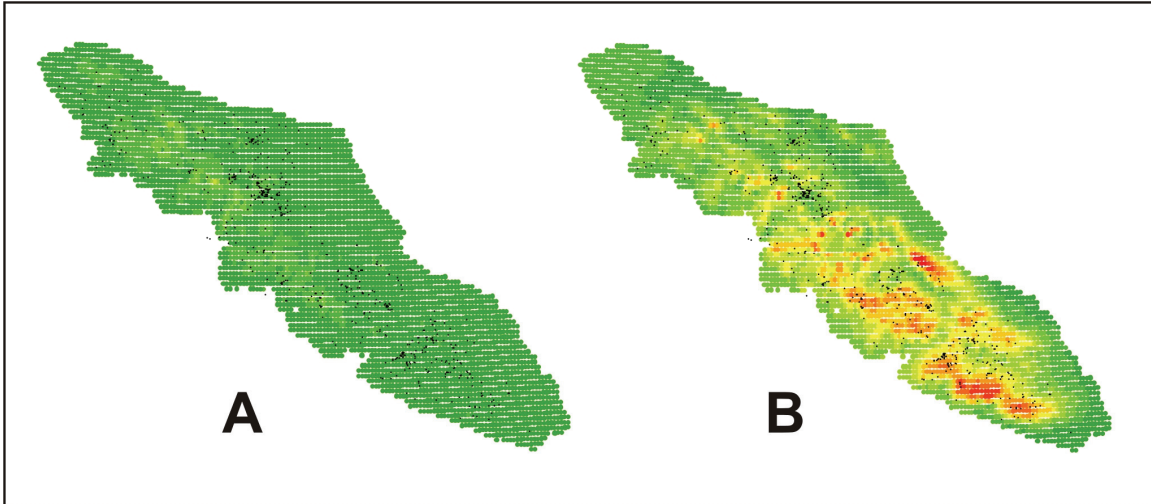
Figure 6.6. Surface rainfall plots for Vancouver Island from the MM5 numerical weather prediction model. A: Precipitation November 14 th , B: Precipitation November 15 th ; dark green = <20mm of rain, and increases to >200 mm (red) in 20 mm increments.
