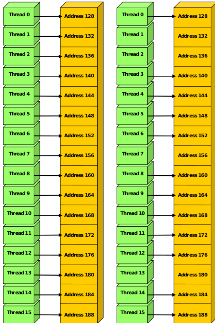
Left: coalesced float memory access, resulting in a single memory transaction. Right: coalesced float memory access (divergent warp), resulting in a single memory transaction.
