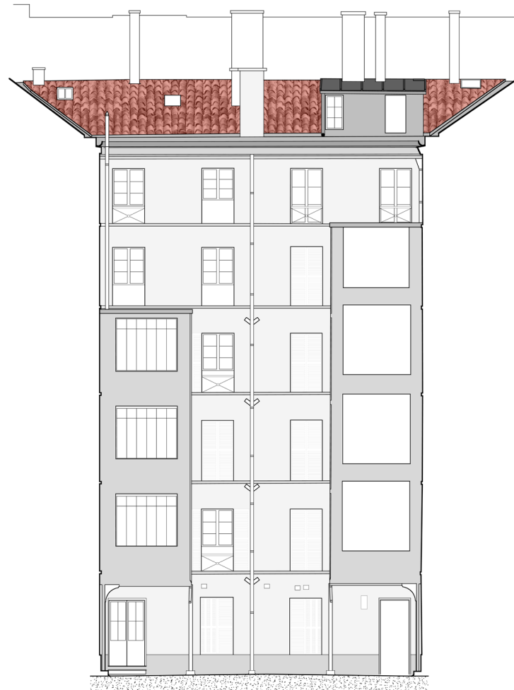
7.20 Courtyard façade looking south. The two wings in the corners will be demolished. NTS
