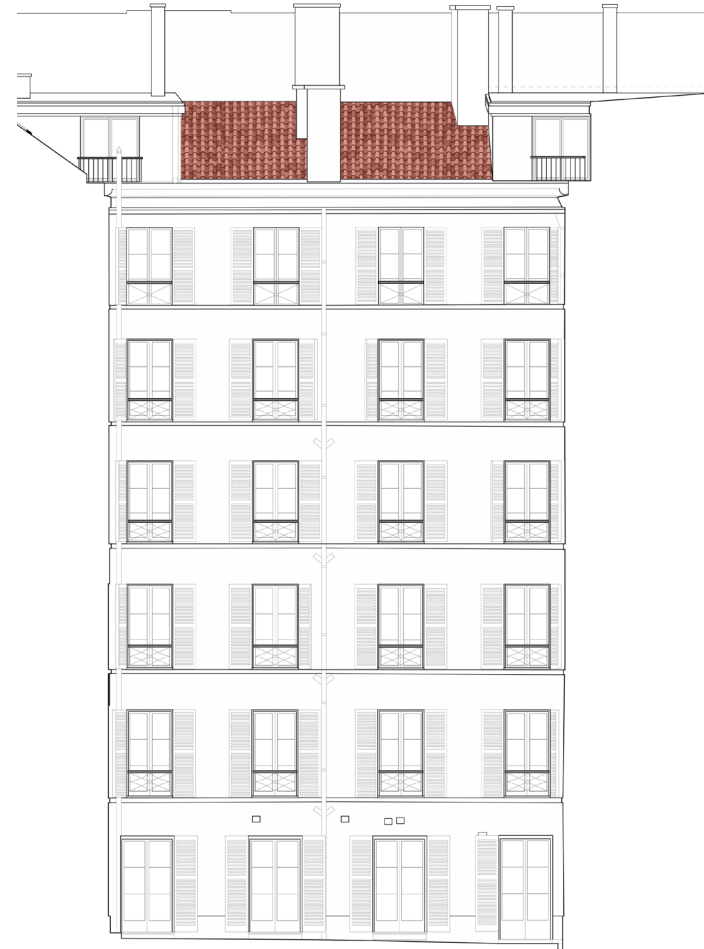
7.34 Proposd courtyard façade looking south. The original openings restored as windows. Ground floor windows to become doors. NTS
