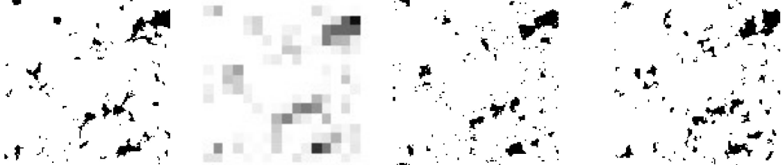
(a) Original images (b) Measurement (c) Reconstruction using Ising model (d) Reconstruction using histogram model
