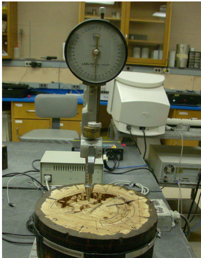
Figure 6.17: Penetrometer tests for new (a), aged and decayed (b) red pine poles
