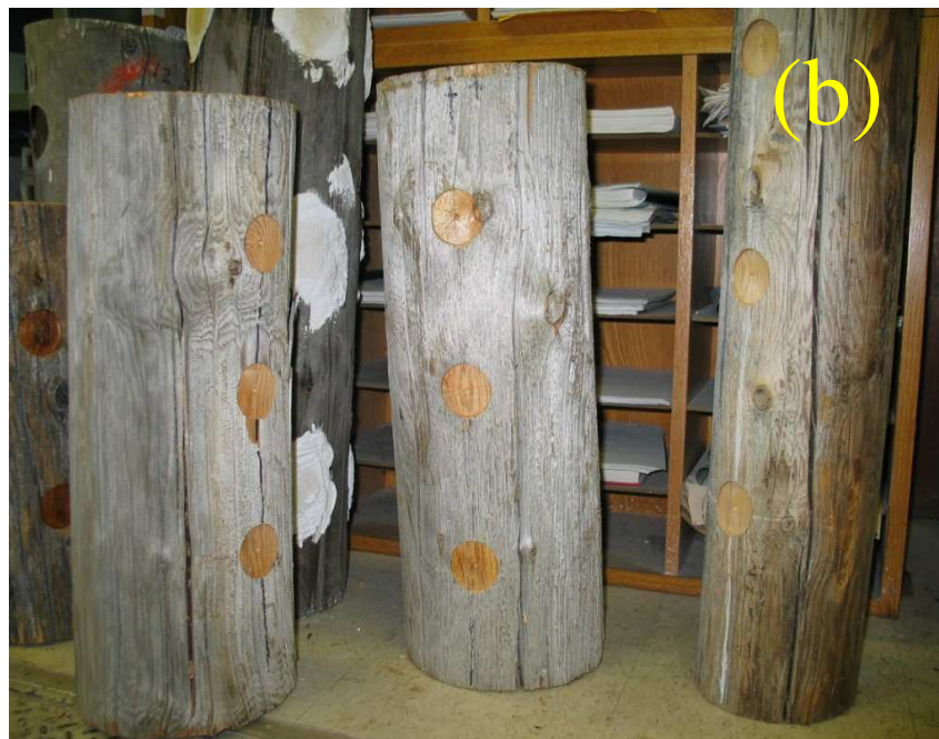
Figure 4.48: Ultrasonic tests in cross-sections of red pine poles: a) new red pine, b) aged red pines (sound)
