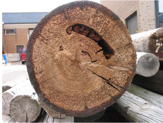
(b) Circumferential decay inside the pole section
