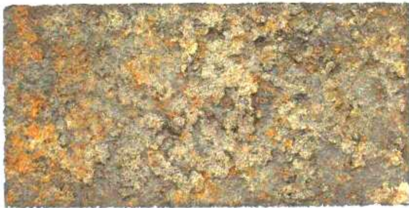
Figure 3.9: “Old steel” specimen with heavy corrosion (old steel)
