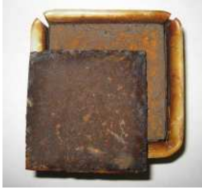
Figure 4.15: Specimen O0W1, after removal from tester, with rust layer detached
