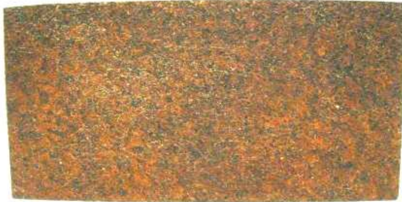
Figure 3.10: “New steel” specimen with light corrosion (new steel)
