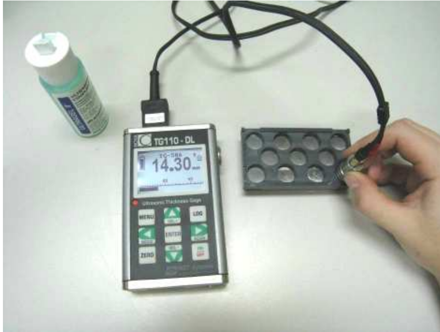
Figure 3.12: UT measurements with templates
