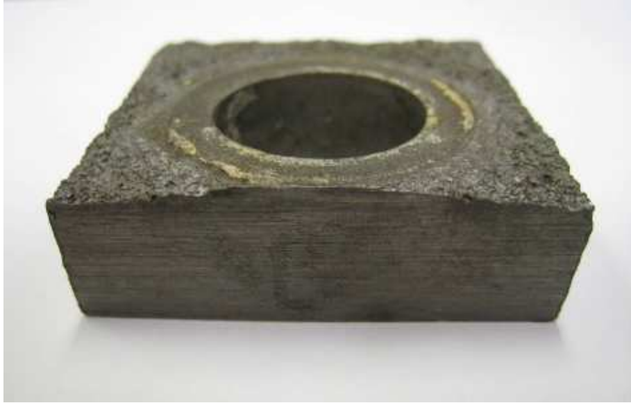
Figure 3.20: Bolt hole specimen (old steel)
