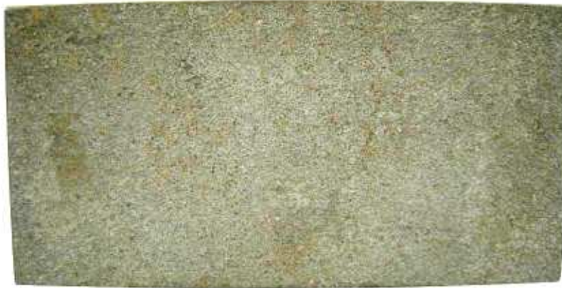
Figure 3.14: Pickled specimen with light corrosion (new steel)
