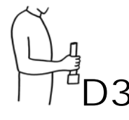
Figure E5-5: Simplified parts with force and moment feedback: Radiator hose attachment simulated with a vertical 35mm handle fixed to a force transducer
