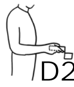
Figure E5-4: Simplified parts with force and moment feedback: Radiator hose attachment simulated with a horizontal 35mm handle fixed to a force transducer
