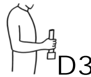
Figure E6-4: Simplified parts with force and moment feedback: Window seal insertion simulated with a 25mm handle perpendicular to the axis of the forearm fixed to a force transducer
