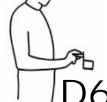
Figure E17-4: Simplified parts with force and moment feedback: Nut rotation simulated with a 25mm handle parallel to the axis of the forearm fixed to a force transducer
