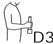
Figure E9- 4: Simplified parts with force and moment feedback: Simulate drill push and torque using with a 25mm handle fixed to a force transducer
