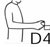
Figure E16-4: Simplified parts with force and moment feedback: Simulate plate hold with a 25mm handle fixed to a force transducer
