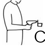
Figure E11-3: Real parts with force and moment feedback: Simulated drill push with drill fixed to a force transducer
