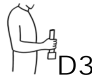
Figure E7-4: Simplified parts with force and moment feedback: Simulate drill hold using with a 25mm handle fixed to a force transducer
