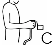
Figure E18-3: Real parts with force and moment feedback: Hose insertion simulated with a hose fixed to a force transducer
