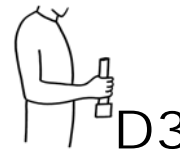
Figure E3- 5: Simplified parts with force and moment feedback: Hammer hold simulated with a 35mm vertical handle fixed to a force transducer
