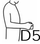
Figure E19-4: Simplified parts with force and moment feedback: Nut rotation simulated with a 25mm handle parallel to the axis of the forearm fixed to a force transducer
