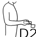
Figure E3- 4: Simplified parts with force and moment feedback: Hammer hold simulated with a horizontal 35mm handle fixed to a force transducer
