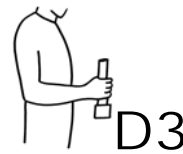
Figure E8-4: Simplified parts with force and moment feedback: Simulated drill push with a 25mm handle fixed to a force transducer
