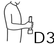
Figure E12-4: Simplified parts with force and moment feedback: Simulate drill push and torque using a 25mm handle fixed to a force transducer
