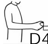
Figure E14-4: Simplified parts with force and moment feedback: Simulated wire harness push with a 25mm handle fixed to a force transducer
