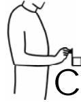
Figure E17-3: Real parts with force and moment feedback: Nut rotation simulated with a nut fixed to a force transducer
