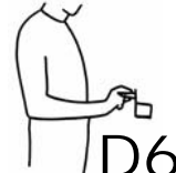
Figure E19-5: Simplified parts with force and moment feedback: Nut rotation simulated with a 25mm handle perpendicular to the axis of the forearm fixed to a force transducer
