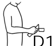
Figure E3- 3: Simplified parts with force and moment feedback: Hammer hold simulated a 35mm handle fixed at 45° to a force transducer
