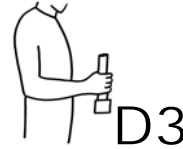
Figure E10-4: Simplified parts with force and moment feedback: Simulate drill hold using a 25mm fixed to a force transducer
