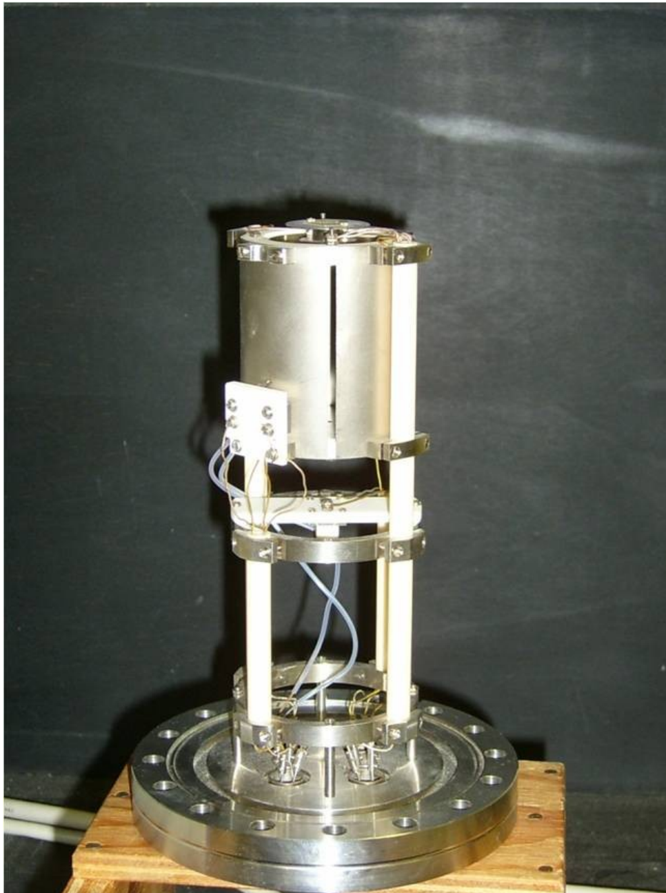
Figure 2.4: An FT-ICR cell showing the pairs of receiver, transmitter and axial trapping plates which constitute the cylindrical shape. The small plate mounted on top of the trapping plate has a platinum grid at the centre, allowing for injection of ions from an external ion source, and a similar assembly exists on the underside to permit EI.
