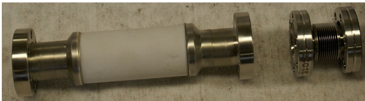
Figure 6.7: Insulated (35 kV) CF feed-through and bellows used to house the HTC and create a junction between the GCR ( \sim 800 Torr) to the SB ( \sim 10 Torr). The junction connecting the two regions is suspended in a high vacuum ( \sim 10^{-7} Torr) region of the mass spectrometer. Reactant gas is only permitted to enter the SB by the HTC.
