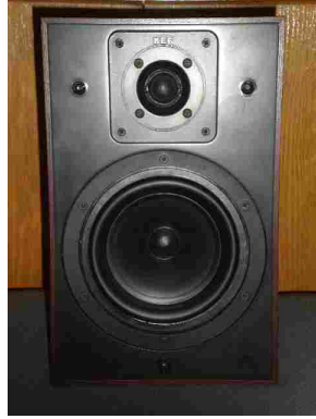
Figure 3.4: KEF two-way loudspeaker. Grill was removed to show the tweeter (3 cm diameter) and woofer (13 cm diameter) units.
