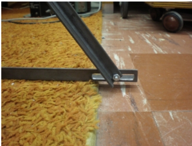
Figure 4.8: The slot in the base of this floor support is attached to the bottom of the angled bar. This may be adjusted so that the bottom of the angled bar is closer to the sheet, increasing the contact between the sheet and surface.
