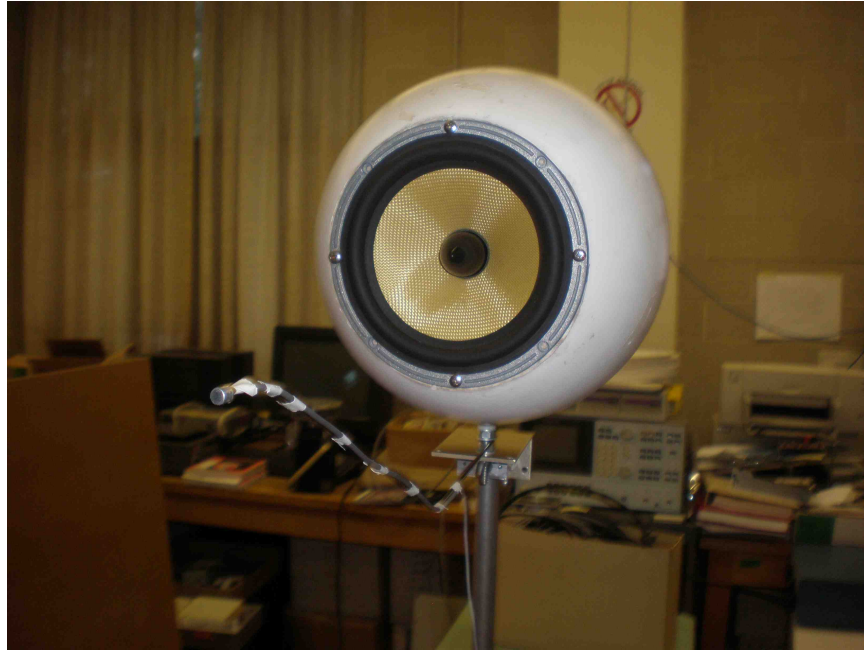
Figure 3.48: Loudspeaker-microphone arrangement for the surface pressure method. A small electret microphone is fixed to the loudspeaker support by a thick, steel support wire. The loudspeaker-microphone distance is then fixed to 28 cm.
