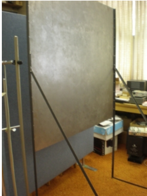
Figure 4.4: Angled view of steel sheet setup. This photograph shows the complete construction of the setup. Vertical supports hold the sheet at a particular height. Angled bars go from the middle of the sheet to the floor for increased support.
