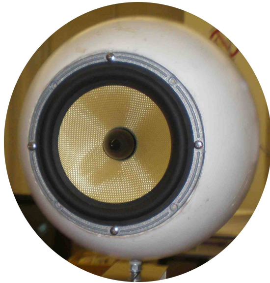
Figure 3.29: Spherical enclosure loudspeaker. A 15 cm diameter driver in a spherical enclosure.
