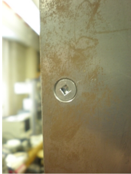
Figure 4.6: A view of the back of the steel sheet showing countersunk fastening. This allows bolts to be inserted flush with sheet surface and therefore, does not reduce the amount of contact between the sheet and the surface under study.
