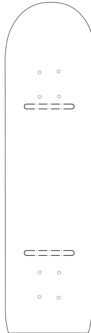
2.12 | Skateboard Stool, assembly drawing showing router cuts
