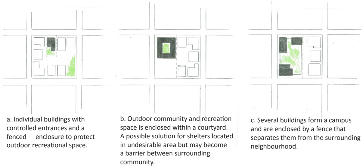
Fig. 2.13 BUILDING LAYOUT The required program can adapt to any of the following forms on the site.
