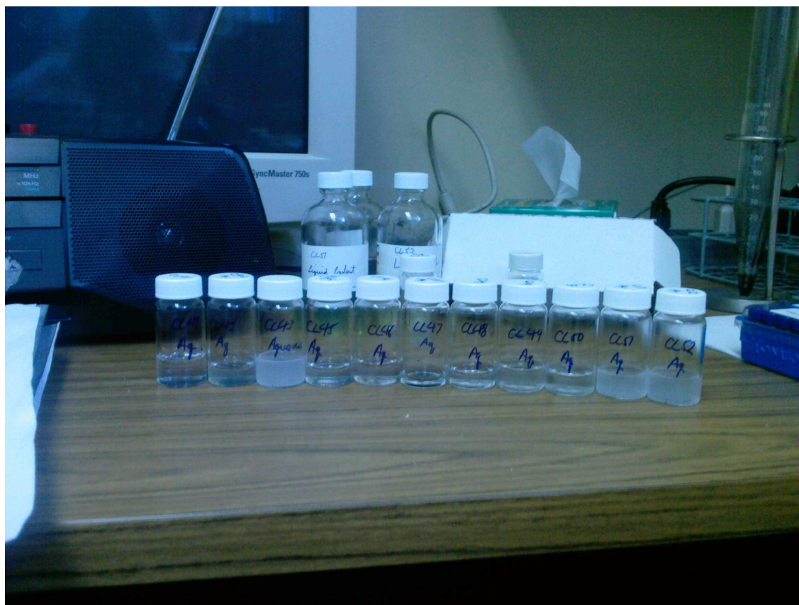
Figure 6.3.5. 1: Recovered Aqueous Phase (600 psig, 4.0°C/min, 2 hrs, 10 ml H 2 O, 100 ml toluene, 78.0 mmol NAPH, 1.50 mmole Mo; 0.91 mmole each (V, Ni), 1500 rpm impeller speed)
