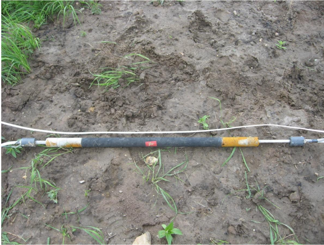
Figure 3-6: RST Packer used in ISATF Injection Wells.
