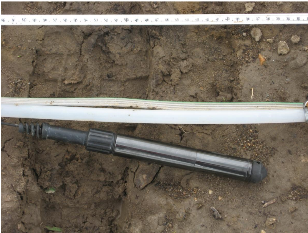
Figure 3-7: Schlumberger CTD Diver connected to direct read cable used in ISATF Injection Wells.
