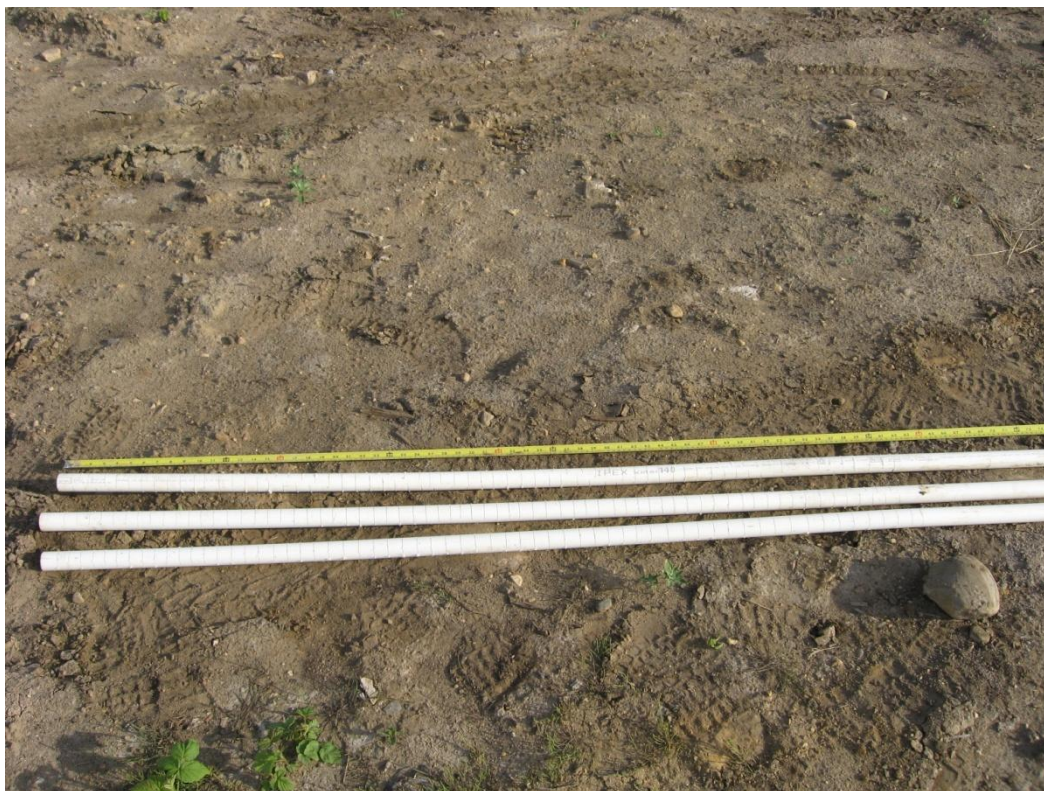
Figure 3-3: Hand-slotted 1-Inch PVC well screens used at monitoring well nest STP-08-159A.
