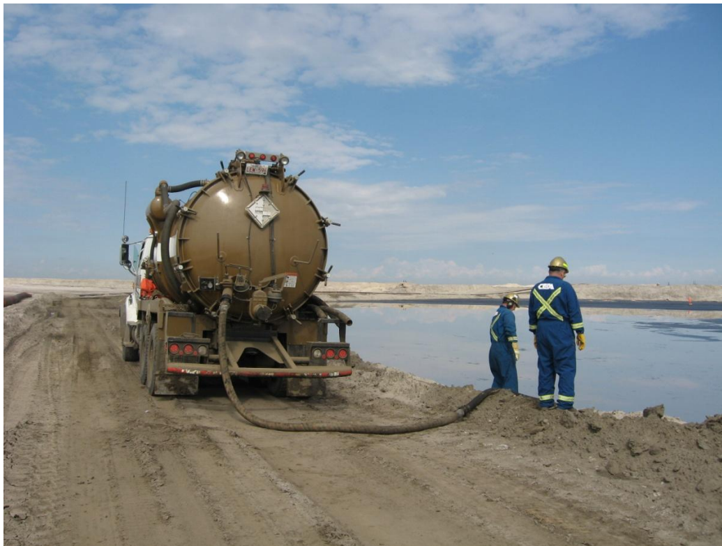
Figure 3-11: Withdrawal of process-affected water from the South Tailings Pond via vacuum truck.
