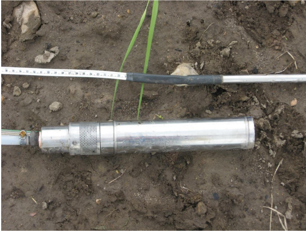
Figure 3-8: Grundfos Redi-flo 2 Submersible Pump used in ISATF Injection Wells.
