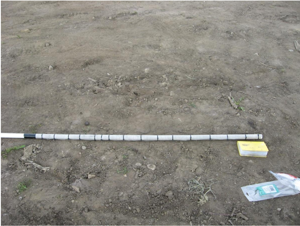
Figure 3-4: Hand-slotted 1-Inch PVC well screen wrapped with filter fabric.
