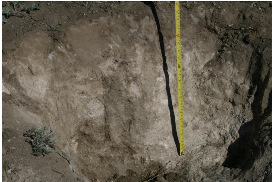
Figure 4.3: Site #21 (Rd 602 01), also within the Buffalo Corridor. Only one till was exposed. Based on field observations (no jointing or staining) and local boreholes, this is Battleford Till at this location.
