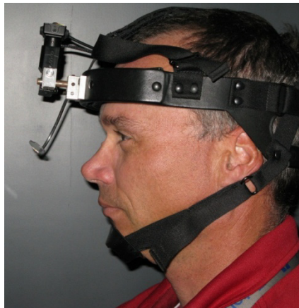
Figure 5-2 – ASL Eye-Trac 6000 mounted on a custom headband
