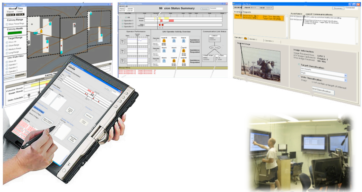
Figure 6. Experimental Platform (from Top Left: Map Display, Mission Status Display, Remote Assistance display; Bottom left: Mission Commander Interface)
