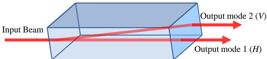
Figure 3.4: (Color online) Calcite Beam Displacer. This type of polarizing beamsplitter, made from a single block of calcite, cut for the maximum walkoff angle between orthogonal polarizations of a normally-incident beam, separates the beam into two spatially separated but parallel output beams in output modes 1 and 2. Note that if both output beams are in the horizontal plane, as shown here, then it is the vertical output which is deviated.
