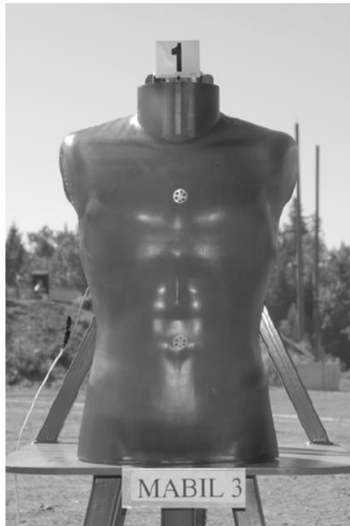
Figure 2.22 - MABIL thoracic surrogate [Ouellet, 2008b]
