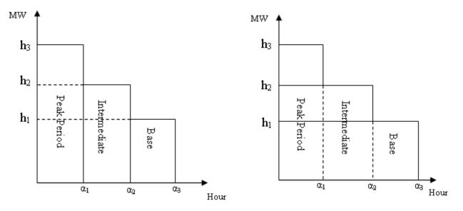
Figure 4-4: Vertical and Horizontal Approximation of Annual Load Duration Curve
