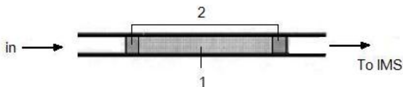
Figure 4.4 Schematic of sorbent trap (1) sorbent material; (2) stainless steel spring stoppers.
