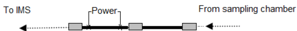
Figure 4.10 Schematic illustrating the two sorbent traps connected in series for breakthrough determination.
