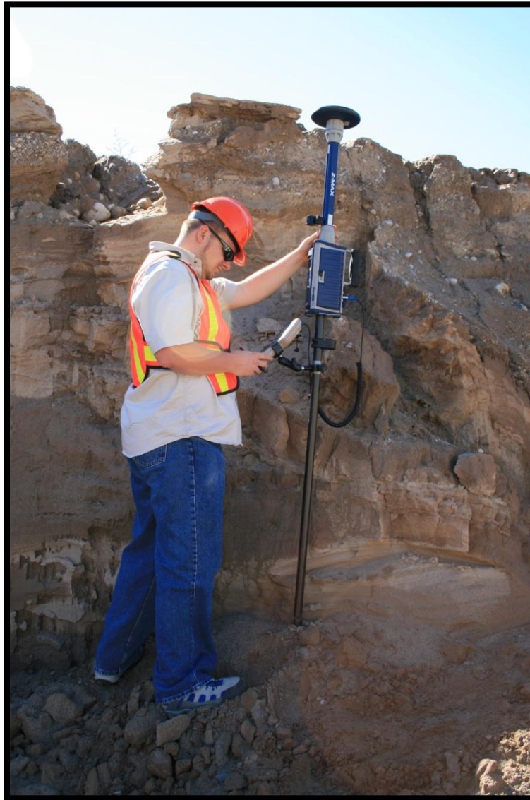
Figure 3-3: The rover unit for the GPS survey system with an attached Allegro computer controller
