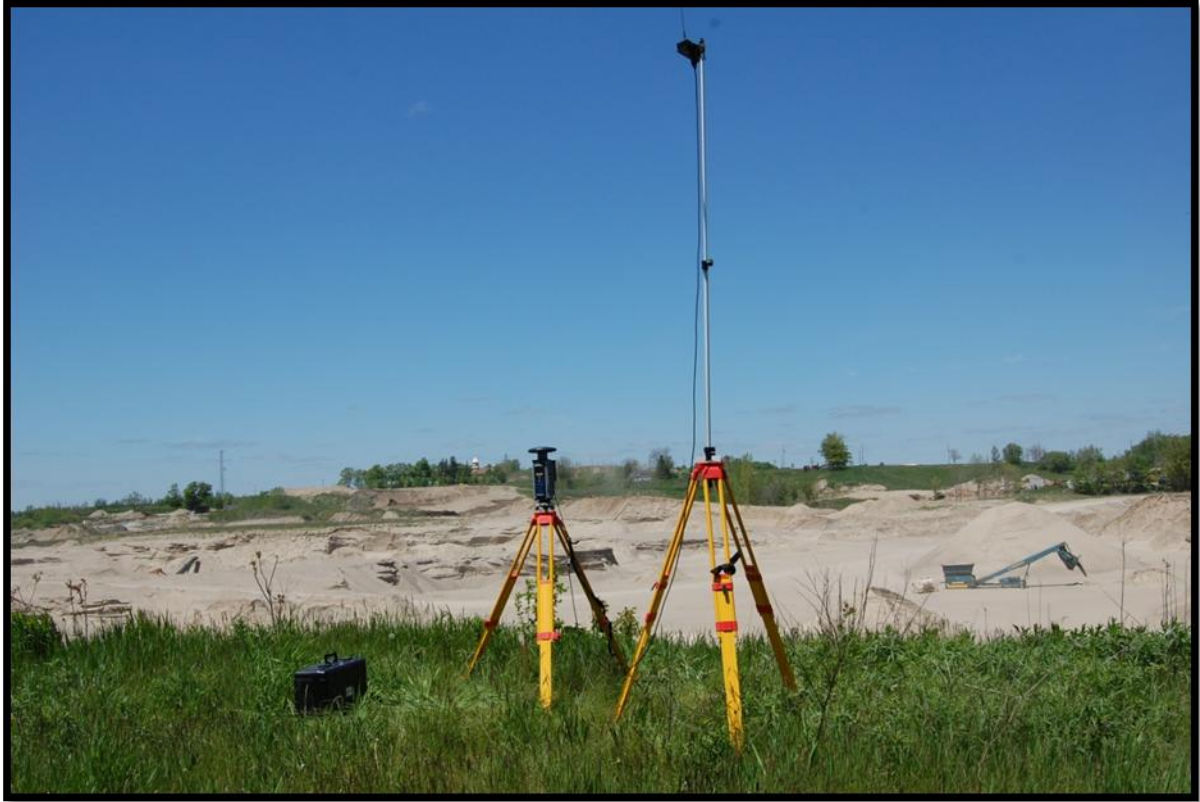
Figure 3-2: Setup of the RTK GPS station, a Thales Navigation Z-Max GPS survey system
