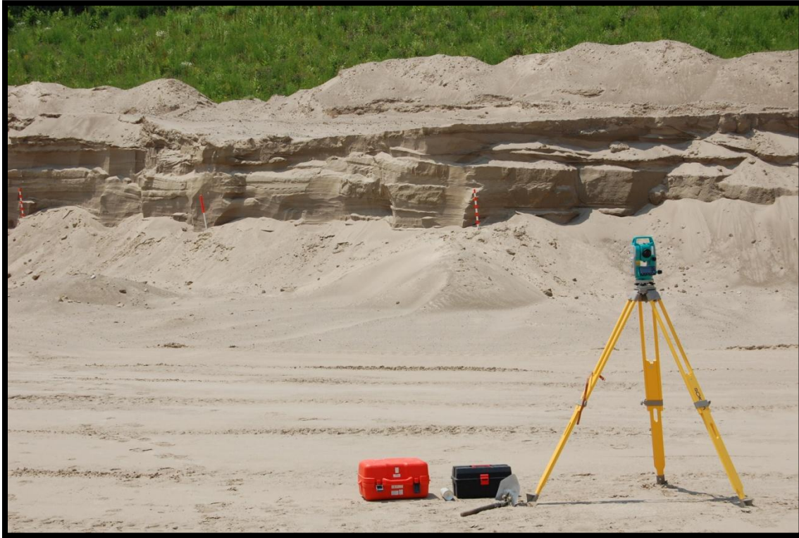
Figure 3-4: A total station setup and ready to take measurements of a section
