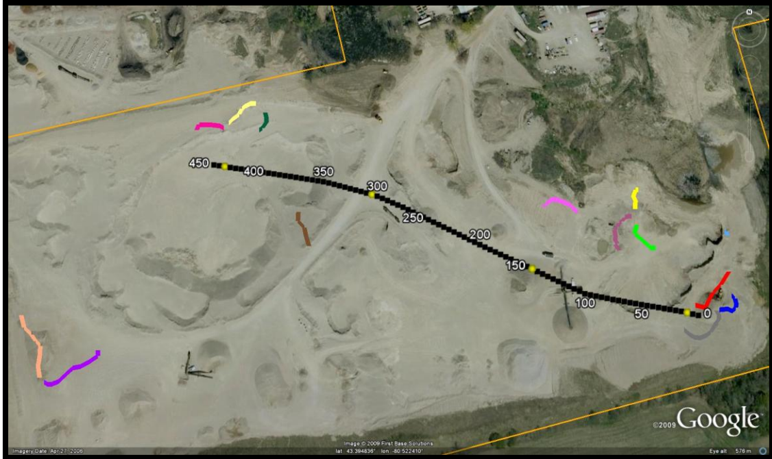
Figure 4-13: The GPR profile path, with position markings, (black) and CMP locations (yellow) linking the subsurface stratigraphy of the studied sections (colours)
