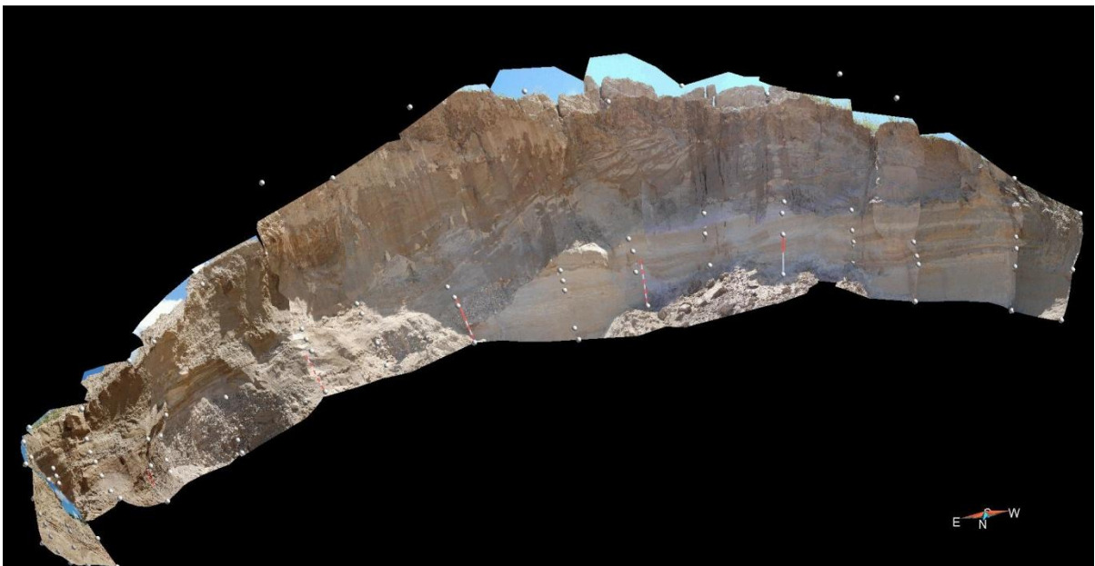
Figure 3-10: An example of a completed section with the images draped onto the surface
