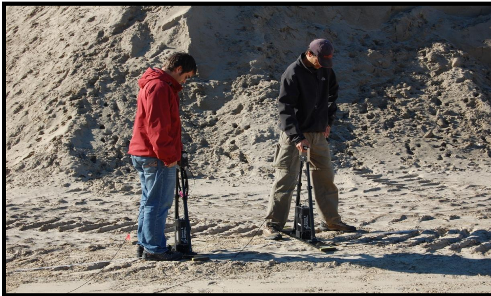
Figure 3-5: Conducting the GPR profile using a PulseEKKO 100A unit with 100MHz antennae
