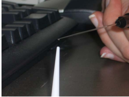
Figure 2-3: Transfer of tear sample from capillary tube to the Advanced Instruments Model 3100 Nanolitre Osmometer sample loading tip.
