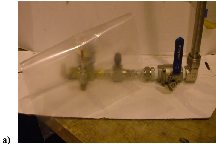
Figure 34: Photo of the equipment used to a) fill the gas bag with air and b) supply nitrogen from an adjacent FCATS to the anode.
