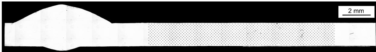
Figure 3.16: A polished specimen with an indented surface showing the grid pattern used for microhardness mapping. The image was taken at \times 50 magnification.
