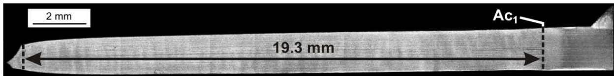
Figure 4.19: A longitudinal section of a fractured weld tensile specimen that had a BM failure location. (Low heat input weld).
