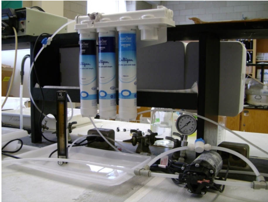
Figure 3-3: Culligan® Aqua-Clear® (model RO30) drinking water system.
