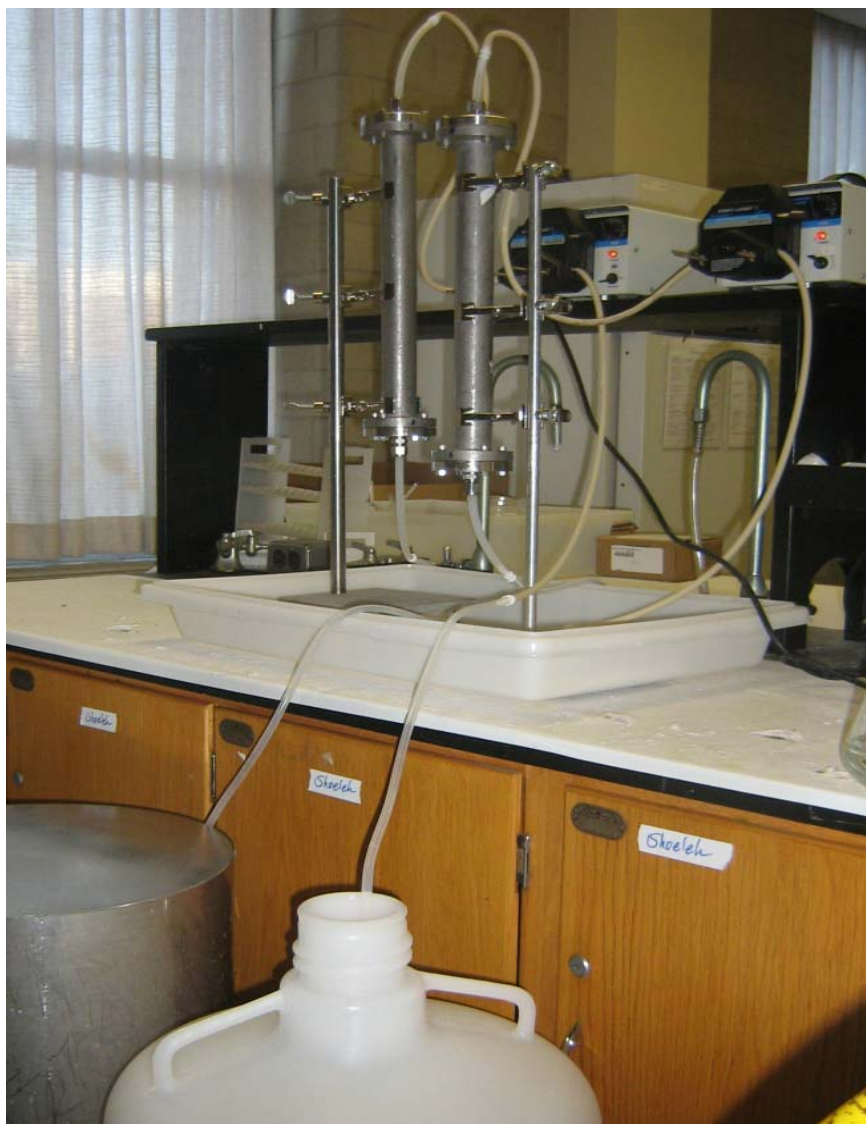
Figure 3-2: IX bench-scale nitrate removal set-up.
