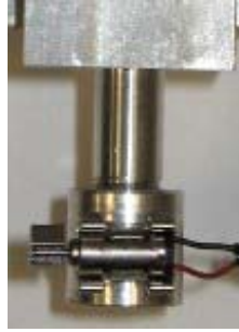
Figure 5-4: Installed Miniature Motor on the Insertion Cap
