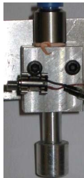
Figure 5-5: Installed Miniature Motor on the Insertion Rod
