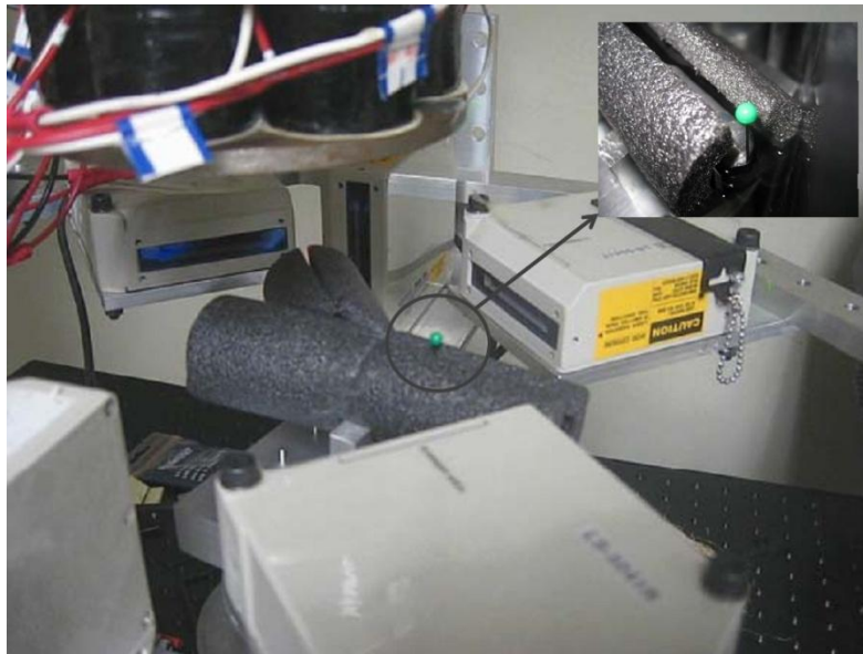
Figure 65 – Capsule robot manipulation in esophagus model
