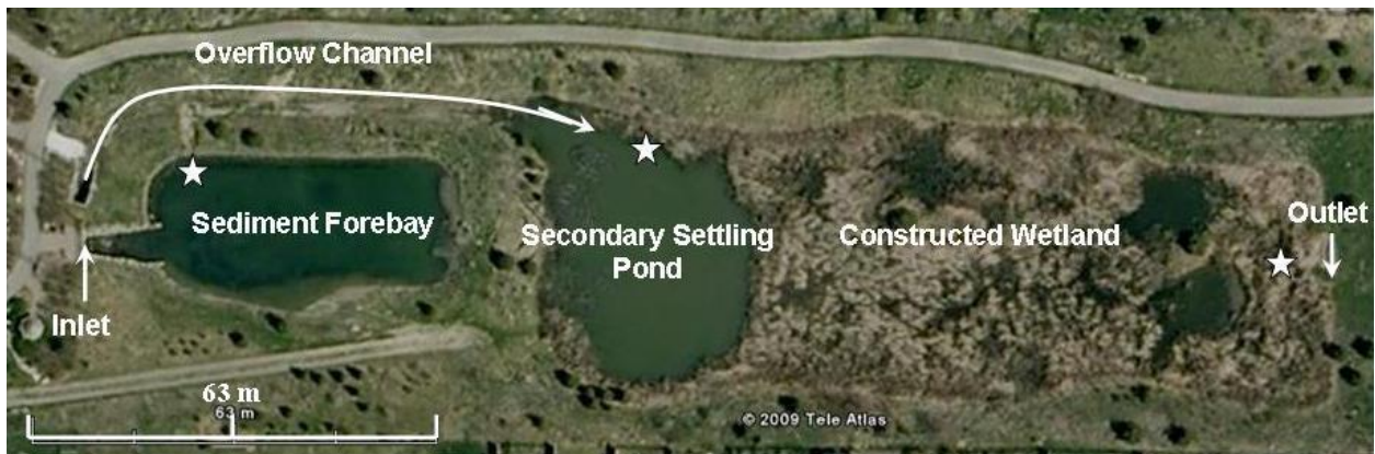
Figure 3. Aerial photograph of Pond 33. Note: The stars represent the approximate locations of PWP installation.
