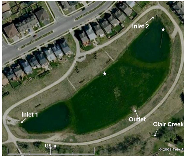
Figure 4. Aerial photograph of Pond 45. Note: The stars represent the approximate locations of PWP installation.
