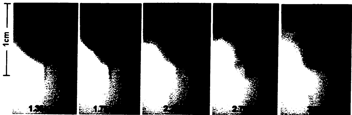
Figure 4.16. Evolution of structural envelope through resonance to destabilisation at medium intensity ( \sim 1.5 \times 10^5 \text{ w/cm}^2 ) in 100% glycerol using a mechanically chopped beam.
