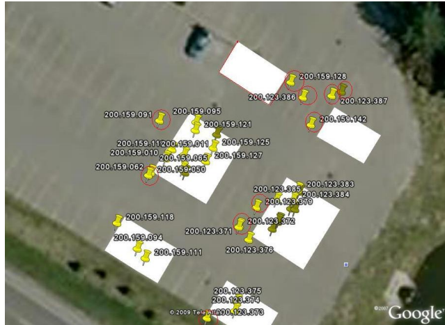
Figure 5.17: Sample data with some of the observations having a relative location outside the allowed boundaries (BIM)
