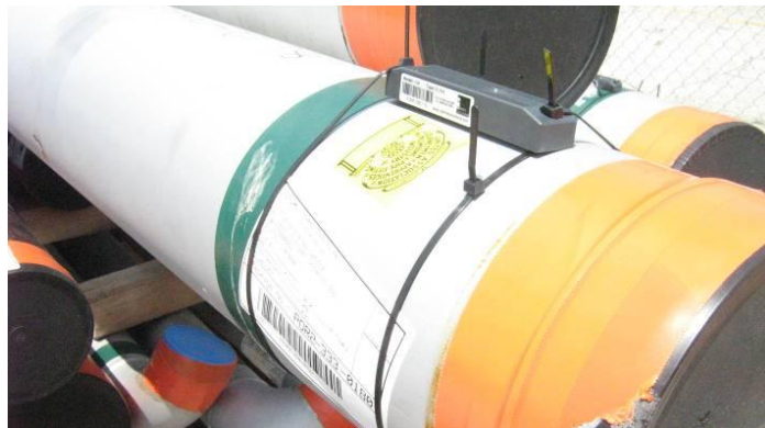
Figure 3.12: A sample of tagged pipe spools
